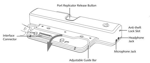
Figure 4-12. Port Replicator front panel
